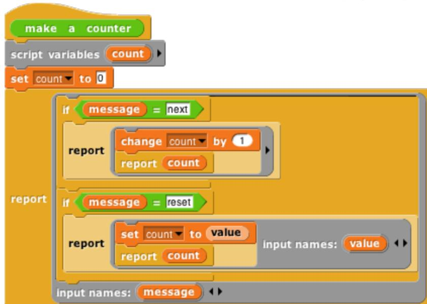
Again, the **make a counter** block represents the **counter** class, and again the script creates a local variable **count** each time it is invoked. The large outer ring represents an instance. It is a *dispatch procedure*: it takes a **message** (just a text word) as input, and it reports a method. The two smaller rings are the methods. The top one is the **next** method; the bottom one is the **reset** method. The latter requires an input, named **value**.
